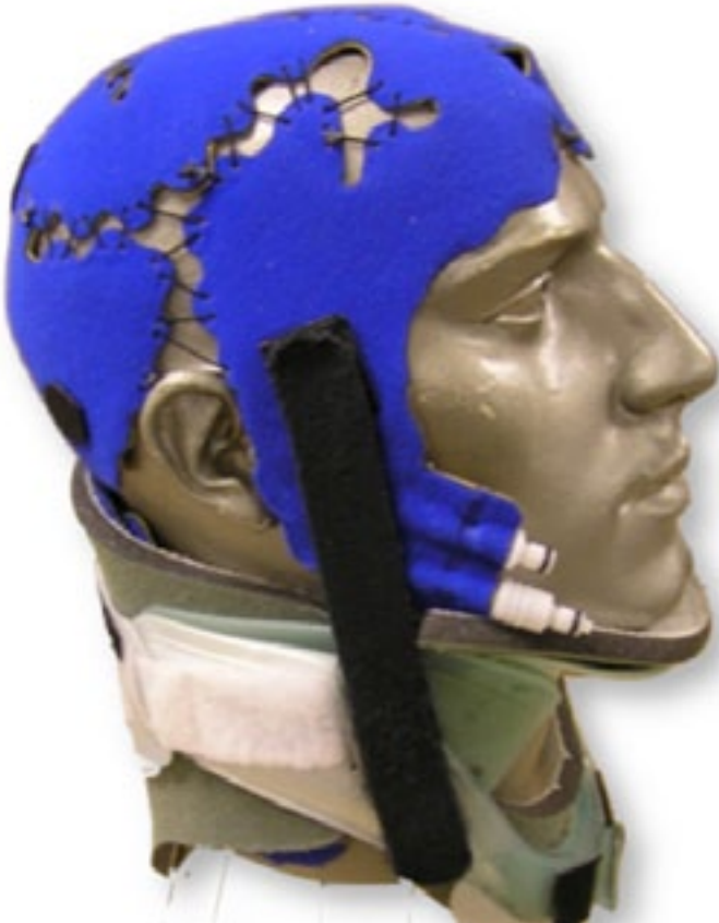
A cooling helmet developed as a spin-off from NASA technology will soon be ready for experimental testing at Beckman’s Biomedical Imaging Center and in the field. Image courtesy John Wang.
